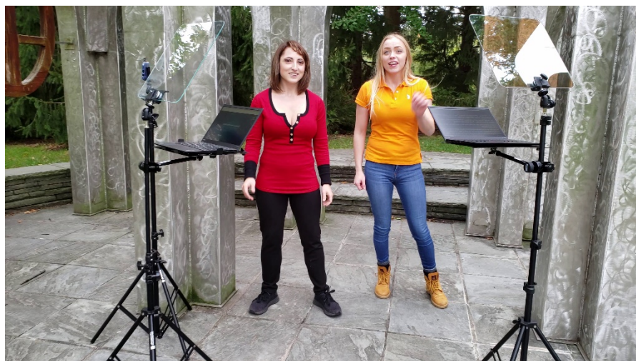
Standard teleprompter glass (left) vs outdoor glass (right).
